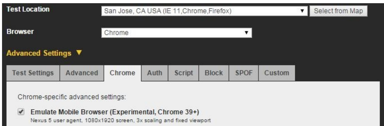
Figure 6-1. The option to enable mobile emulation is found on the Chrome tab of the Advanced Settings section. This will cause desktop Chrome to masquerade as a Nexus 5 and compel the server to produce the mobile web version of the test page.
