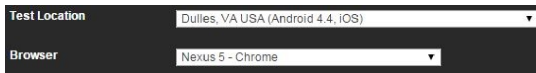
Figure 6-5. Testing on a native device is as straightforward as selecting a mobile-supported location and picking your device
