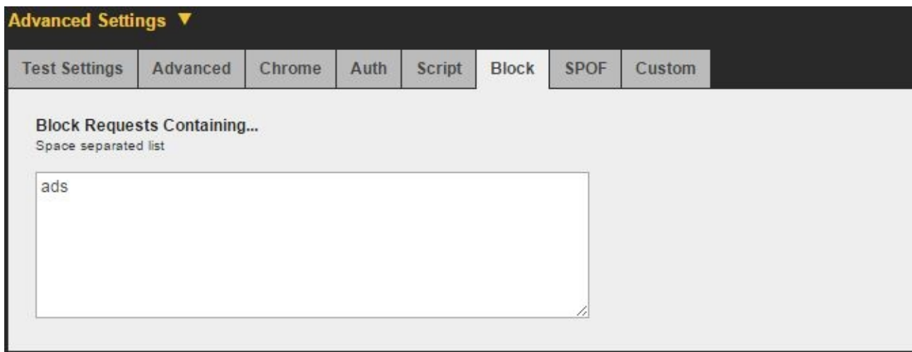
Figure 8-7. The block tab takes a space-delimited list of substrings to be matched against blocked requests. If the request URL contains any of these substrings, it will be prevented from materializing.
