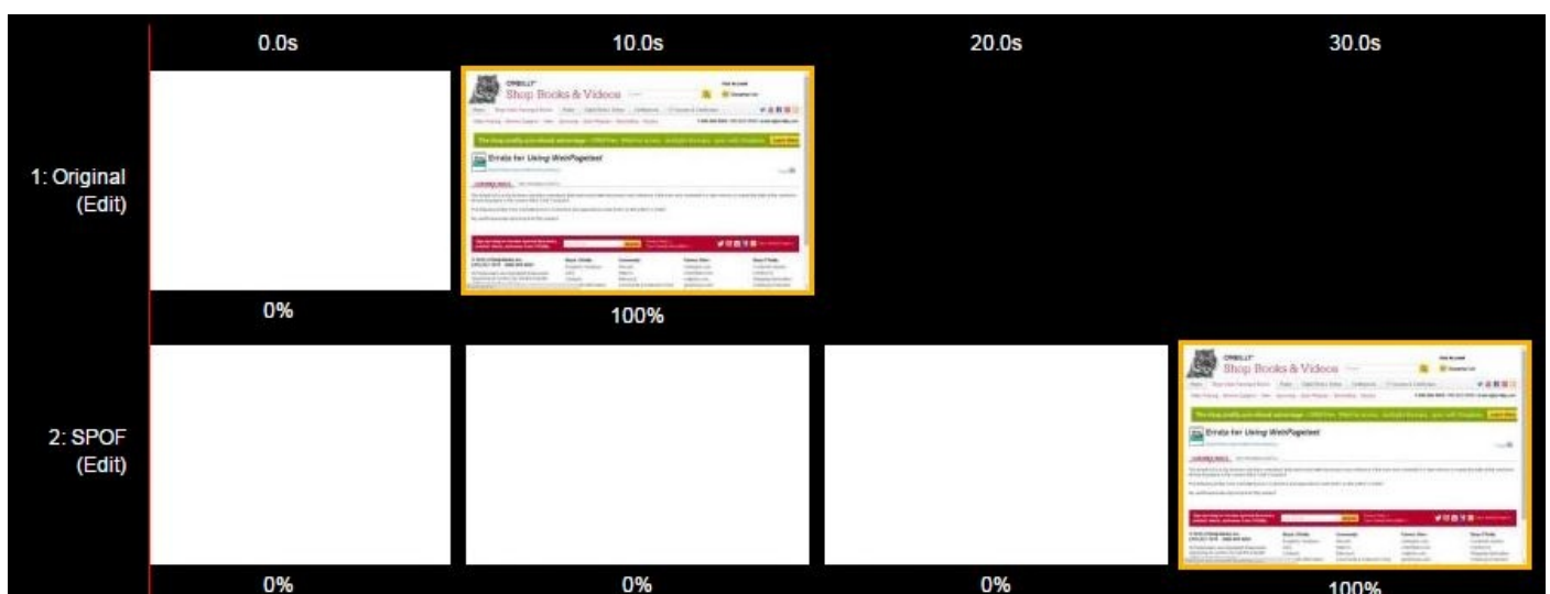
Figure 8-4. The SPOF tab generates a comparison of tests with and without domain failures. The filmstrip view clearly shows the page-load impact of SPOF in which the SPOF page takes more than 20 seconds longer to load.
