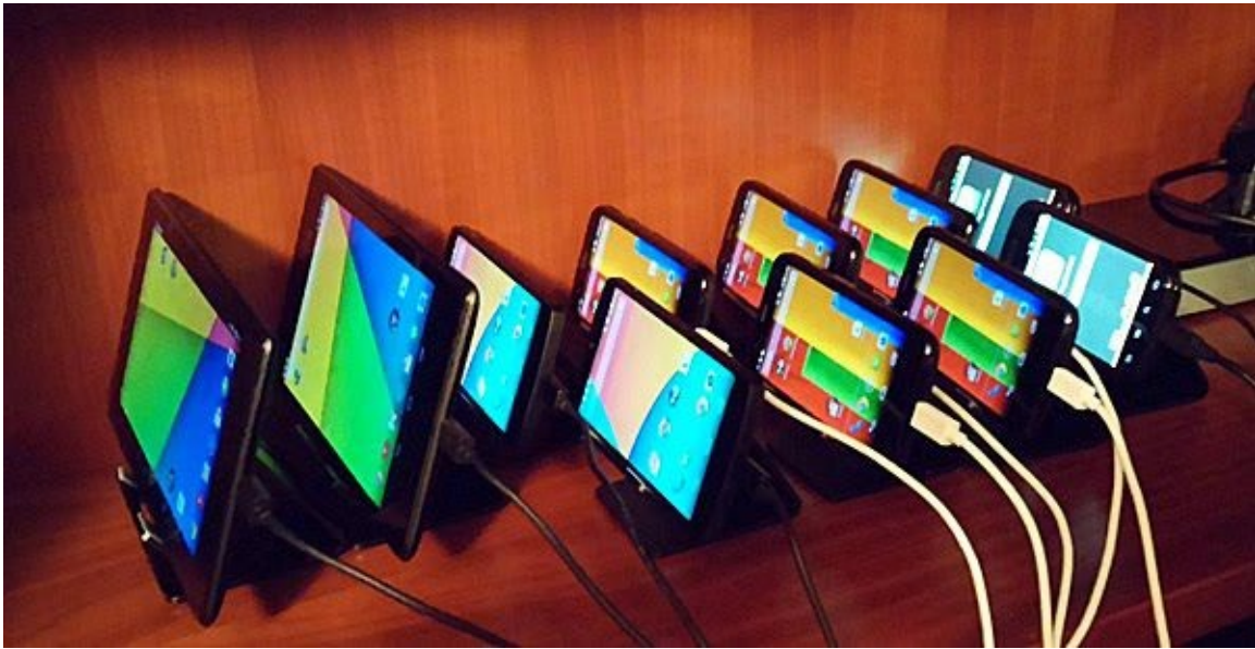
Figure 6-6. In this 2014 photo, the actual Android devices hooked up to the WebPageTest agent in Dulles, Virginia are shown. From left to right: Nexus 7 (landscape), Nexus 7 (portrait), two Nexus 5, five Motorola G, and two Motorola E. Source: Android web performance testing takes a big leap forward
