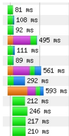
Figure 2-12. An example of a series of requests in a waterfall with tall and narrow slope. Many requests are initiated at roughly the same time, as illustrated by their mostly aligned left edges.
