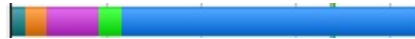
Figure 2-6. An example of a request with all five phases: DNS lookup (teal), initial connection (orange), SSL negotiation (purple), TTFB (green), and content download (blue)
