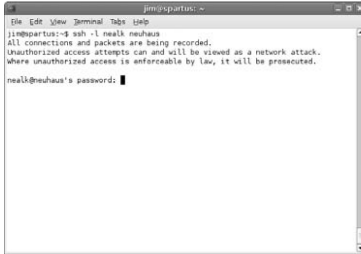
Figure 6-5: A SSH connection showing the /etc/issue.net message
