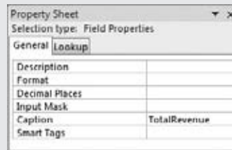
Figure 3-6: Using the Property Sheet dialog box for field properties is an alternate way of defining an alias for your field.
