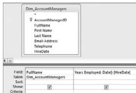
Figure 5-22: You are calculating the difference between today's date and each manager's hire date.
