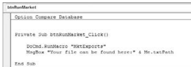
Figure 10-23: When you click the command button, a DoCmd action will run the macro and then call a message box.
