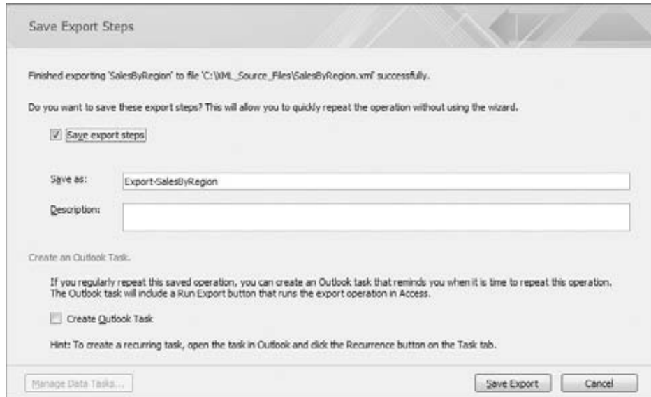
Figure 17-3: You can choose to save your export process so that you can perform it routinely with the touch of a button.
