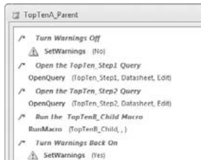
Figure 9-3: The two SetWarnings macro actions will not run in an un-trusted database.
