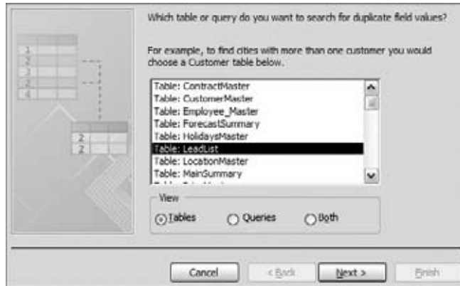
Figure 4-4: Select the dataset in which you want to find duplicates; then click Next.
