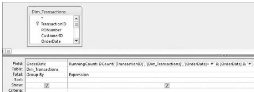
Figure 7-25: This query returns all invoice dates and the number of invoices processed on each date.
