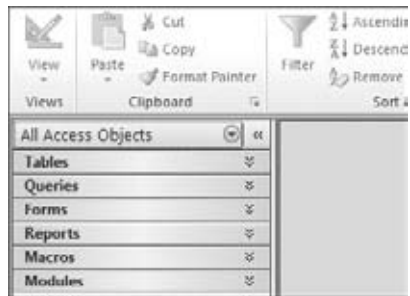
Figure 2-1: The navigation pane on the left allows you to navigate through the six types of database objects: Tables, Queries, Forms, Reports, Macros, and Modules.
