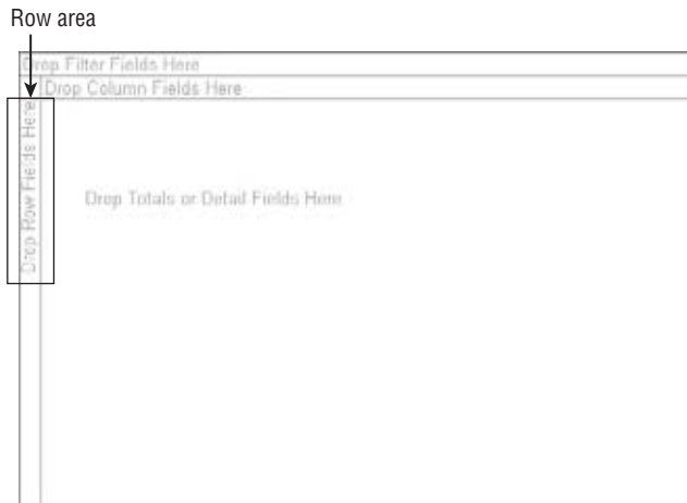
Figure 12-3: The Row area displays values down the left side of the pivot table.
