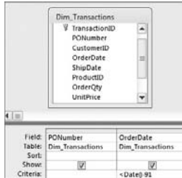
Figure 5-21: No matter what day it is today, this query will return all orders older than 90 days.
