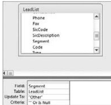
Figure 4-14: This query updates blank values in the Segment field to a value of “Other.”
