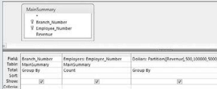
Figure 8-29: Build a query using the Partition function to create a frequency distribution.
