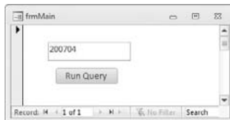
Figure 10-19: Now you can pass your parameters to your query through a form.
