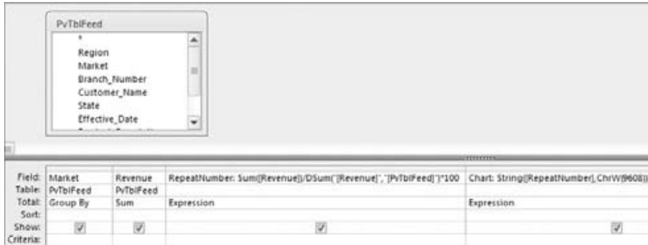
Figure 13-16: Use the DSUM Function to establish a ceiling on your repeat number.
