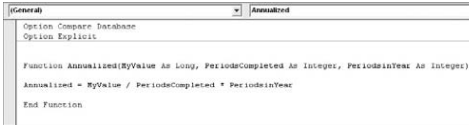
Figure 10-7: This custom function accepts three variables and uses them in an expression.
