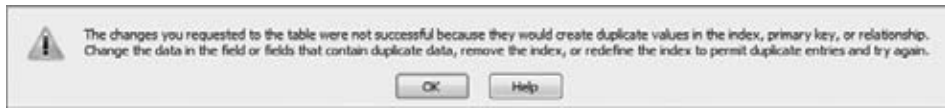
Figure 4-2: If you get this error message when trying to set a primary key, you have duplicate records in your dataset.
