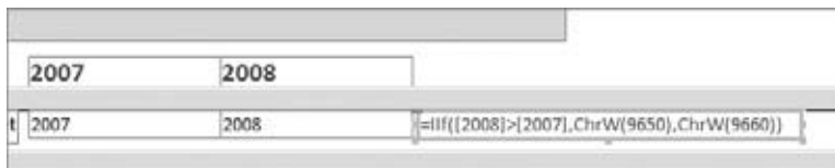
Figure 13-21: Build an IIf statement that evaluates revenue and returns either an up arrow or down arrow.
