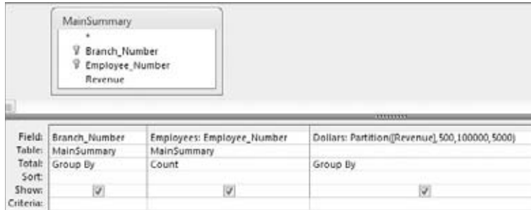
Figure 8-27: This query creates a separate frequency distribution for each branch number in your dataset.
