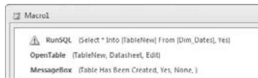
Figure 9-1: This macro runs a SQL statement that makes a new table, opens the new table, and throws up a message box.
