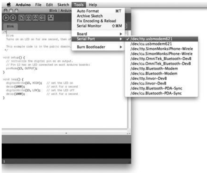
Figure 2-5 Selecting the serial port (on a Mac)
