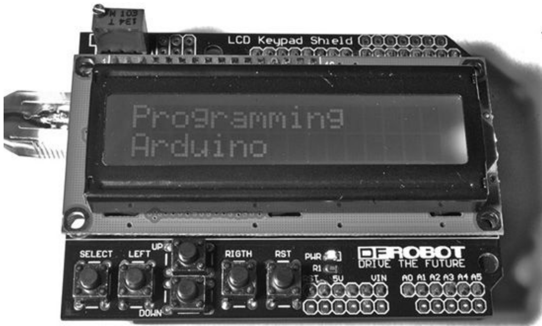
Figure 9-2 LCD shield attached to an Arduino board
