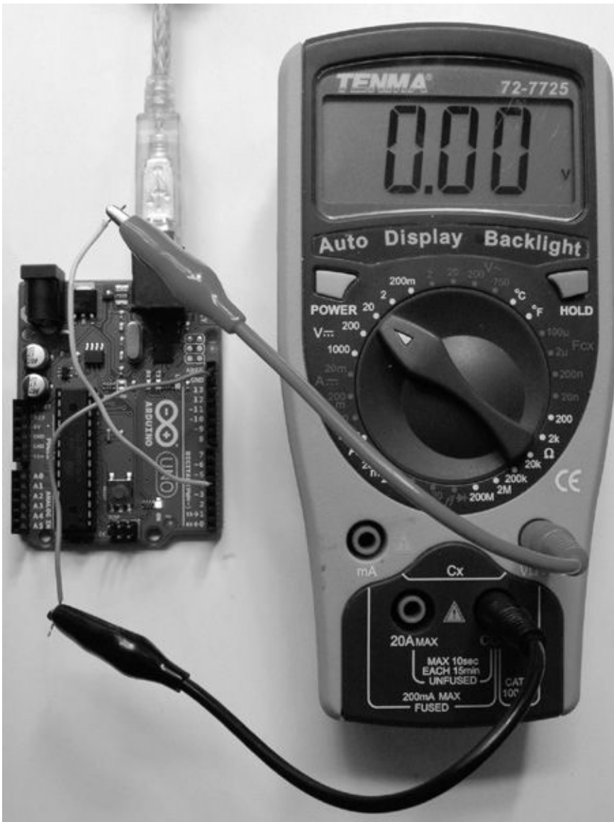
Figure 6-1 Measuring outputs with a multimeter
