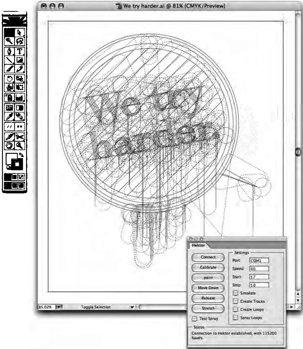
The Scriptographer plug-in for Adobe Illustrator by Jürg Lehni, running the Hektor software that computes motion paths and directly communicates with the hardware. Image courtesy of Jürg Lehni.
