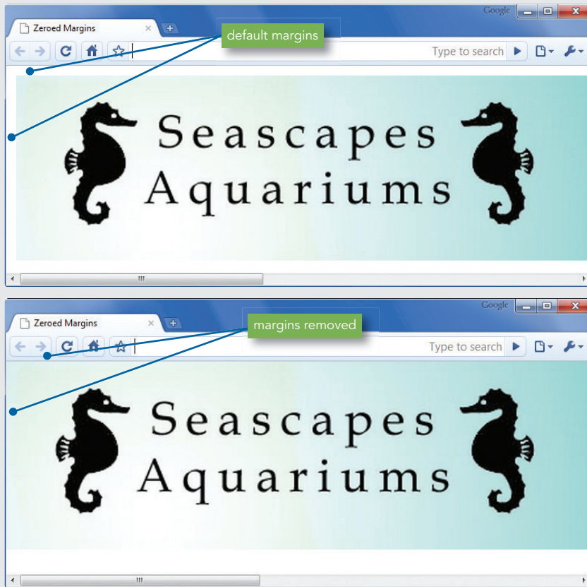
Figure 6-10: Zeroing margins to place images against the edge of the window Seahorses courtesy of www.seascapesaquariums.com
