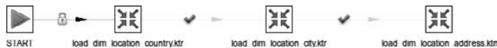
Figure 8-11: The load_dim_location.kjb job ensures top-down level-wise loading of the snowflaked location dimension tables
