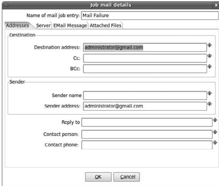
Figure 12-8: The Addresses tab page in the configuration dialog of the Mail job entry
