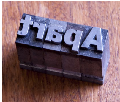
FIG 3.5: Some metal type. The physical dimensions of the metal around the letter make up the em canvas.
