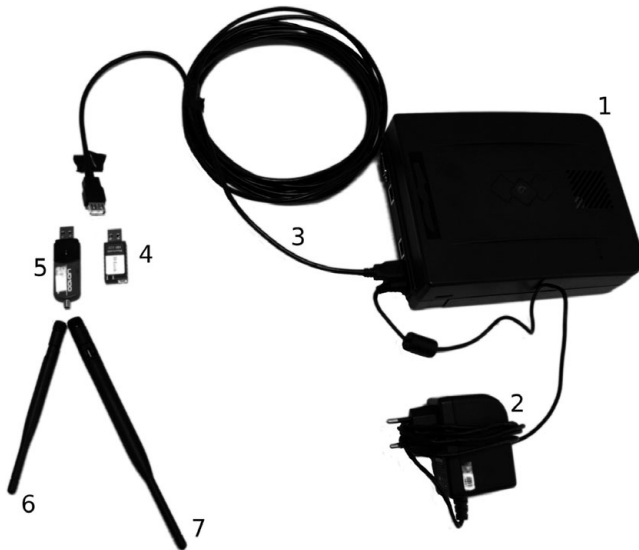
Figure 14.1 Components of a Bluetooth scanner for tracking purposes: computational unit (1), power source (2), USB cable (3), class 2 Bluetooth sensor (4), class 1 Bluetooth sensor (5), and different types of external antennas (6, 7).
