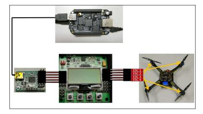
The following is a close-up image of the connections between the servo controller and the flight controller board:
