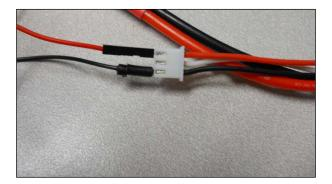
You will connect the control signal of the servos to the GPIO pins of the BeagleBone Black. There are two GPIO pin connectors on the BeagleBone Black, one on each side of the board. They are labeled **P8** and **P9**, but just in case you again need an image with the pin-out, it is here:
