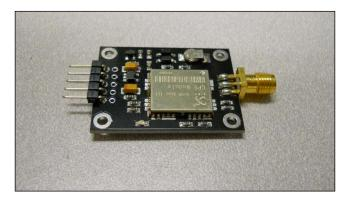
You should also purchase an antenna that can connect to the RF (gold) connector on the board. This is type SMA; these are available from electronic online retailers. Here is an image of a possible antenna:
