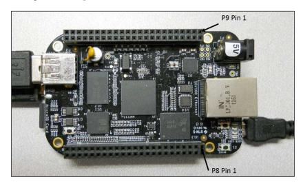
Connect the 5V of the sensor to the P9\_3 on the BeagleBone Black, and the **GND** to P9\_1 on the BeagleBone Black. Connect the **Vo** on the sensor to the **hv** side of your level shifter, and the **lv** side of the level shifter to one of the ADC inputs, for example, P9\_39 on the BeagleBone Black. Connect the **GND** on the level shifter to P9\_2.
