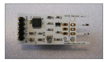
You can mount it to the mast if you'd like. You can perhaps use a small piece of heavy-duty tape and mount it to the top of the mast. However, as you'll see a bit later, it will be useful to be able to turn the sensor in order to do a complete sensing of the wind, so it is useful to mount the sensor to a servo.
