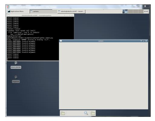
When I first did this, the camera window eventually turned black and did not show the output from the camera. To actually see the image, I needed to change the resolution of the image captured by the USB webcam to one supported by the camera and OpenCV. To do this, you need to edit the camera.py file by adding two lines like this:
