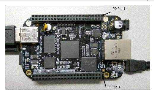
Connect the control wire connection on each servo, normally a yellow wire, to one of the GPIO pins on the BeagleBone Black that supports PWM output. For example, connect P8\_13 and P9\_14 on the BeagleBone Black. You can use P8\_13 and P9\_14 for the two servos in this project. Here is an image of the connections:
