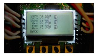
5. The next step is to calibrate the level sensors of the flight controller. From the main menu, select the **ACC Calibration** option as shown in the following image:
