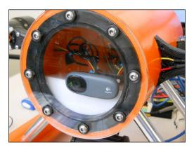
You can also choose a rounded dome of clear acrylic, as shown in the following image. This came from a company called EZ Tops, and it can be ordered online at www.eztopsworldwide.com/smalldomes.htm. You will put it on the end of your ROV, assembled with a gasket and some small bolts. This clear plastic gives you a good view of the underwater world and reduces the drag when moving in the forward direction.
