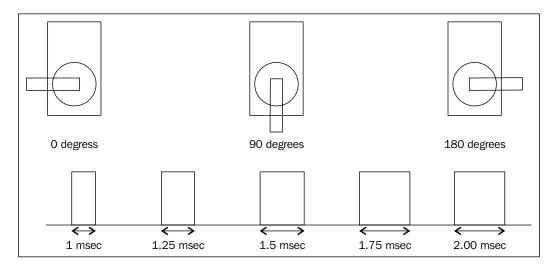
These pulses are sent out with a repetition rate of 60 Hz. You can position the servo to any angle by setting the correct control pulse.
