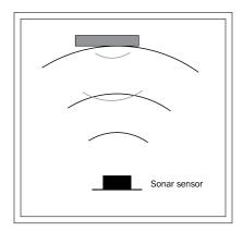
The sensor then measures return of waves, if any. It then uses the time difference between when the sound wave was sent out and when it returns to measure the distance to the object.
