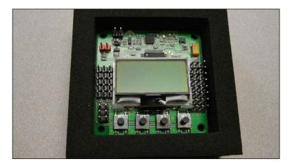
The flight control board takes its flight inputs via a set of input signals that would normally come from an RC receiver to control the quadcopter, and then sends out control signals to the four motor controllers. You'll want a flight controller as it has built-in flight sensors, so it can handle the feedback control for the motors. The inputs from the BeagleBone Black will come in as electric commands to turn, bank, go forward, or increase/decrease the motor speed.
