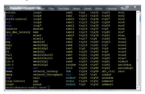
3. The video0 device is the USB webcam. If you see its entry in the directory, then it means the system can access your camera.
