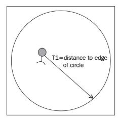
If you have two satellites that send signals and you know the distance between the two, you can draw two circles, as shown in the following diagram:
