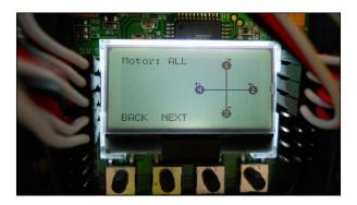
4. Now that the basic quadcopter is configured, you can test the sensors by pressing the **BACK** button until you get to the main menu. Press the **UP** key until you can select **Sensor Test**, as shown in the following image:
