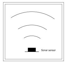
The device sends out a sound wave 10 times a second. If an object is in the path of these waves, then the waves reflect off the object, sending waves that return to the sensor, as shown here:
