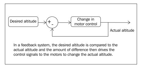
In this case, the desired altitude will be in the middle of the webcam window that captures the colored ball. The actual altitude will be in the center of the color blob in the webcam window. These will be compared and the BeagleBone Black on the quadcopter will adjust the throttle to either increase or decrease the value to compensate for the difference. This is well explained in the preceding diagram.
