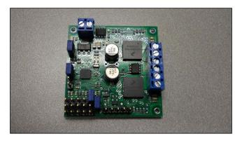
This piece of hardware will convert the USB commands to voltage that controls your motors.
