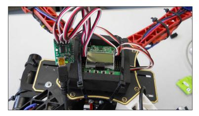
Note that you need to use the foam that came with the flight controller as this will dampen the vibrations inherent in the system so that the sensors can make more accurate readings. Make sure you do not connect power to the servo controller; it does not need to supply power, it just sends the appropriate signals via the servo lines to the receiver input.
