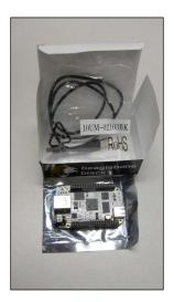
The USB connection not only supplies power to the host computer, but also provides a simple, yet fairly limited, way to communicate with the board. You'll use this USB cable for power, but that's about it.
