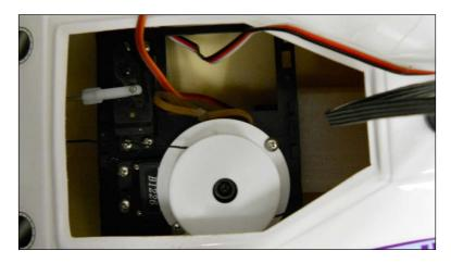
You'll use your BeagleBone Black to control these two servos that will control both the rudder and the sail position, so let's start by connecting these two servos to the BeagleBone Black. You'll drive the two servomotor control signals from the BeagleBone Black GPIO pins, but you'll supply the DC power from a battery.
