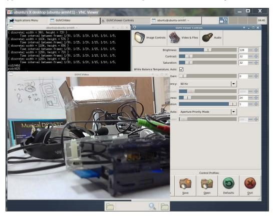
The video window displays the webcam images and the **GUVCViewer Controls** window controls the output from the camera. The default settings may work fine for your USB webcam. However, if you get a black display for the camera images, you will need to adjust the settings. Select the **GUVCViewer Controls** window and then the **Video & Files** tab. You will see a set of selections where you can adjust the settings for your camera:
