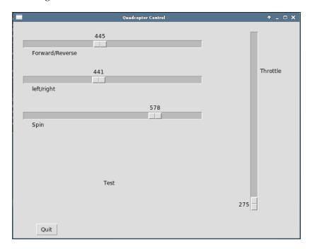
You can use this interface to control the flight controller board. One thing you will need to do (if you have not done previously) is using this interface to recalibrate your ESCs, adjust the stick sensitivity, and the other settings that you might want to tweak on the flight controller board.
