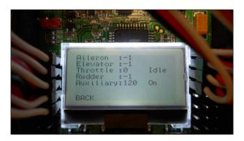
As you run the program and change the values of each servo, you should see that these values also change. For example, if you set the value of servo 0 to 275, the flight controller board should show the aileron set to a value that would turn it left, like this:
