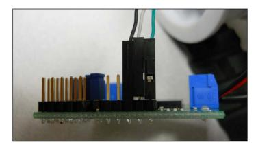
4. Now, there's one more step before you connect the board to the BeagleBone Black. Remove the jumper at the top of the board so that the board will accept serial commands. Here's an image of the jumper, and I like to just turn it sideways so that I don't lose the jumper:
