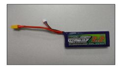
This battery will come with two connectors: one with large gauge wires for normal usage and a smaller connector used to connect to the battery recharger. You'll want to build connectors that can connect to the screw-type connectors of the servo controller. I purchased some XT60 connector pairs, soldered some wires to the mating connector of the battery, and screwed these into the servo controller.
