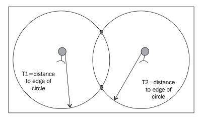
However, you know that since you can only be at points on the circle, you must be at one of the two points that are on both circles. Adding an additional satellite would eliminate one of these two points, providing you with an exact location. You will need more satellites if you are going to do this in all three dimensions. For more information on how GPS works, see http://www.trimble.com/gps\_tutorial/.
