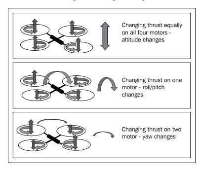
As you can see, controlling the relative speed of the four motors allows you to control the various ways the device can change its position. To move forward, you would want to adjust the pitch so that the quadcopter is tilting forward. Then you'll add some thrust so that instead of going up, the device would move forward, as shown in this diagram:
