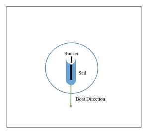
In this case, the diagram shows that the sail is in, and your rudder is in line with the boat. Now let's introduce some wind. If you want to sail with the wind, your boat's rudder and sail should be configured like this:
