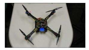
The quadcopter has two sets of counter-rotating propellers, which simply means that two of the propellers rotate one way and the other two rotate the other way to provide thrust in the same direction. This provides a platform that is inherently stable. By controlling the thrust, all the four motors allow you to change pitch, roll, and yaw the device. Here is a diagram that might be helpful:
