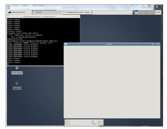
In my case, the camera window eventually turned black and did not show the output from the camera. I realized that I needed to change the resolution of the image to one that is supported by the camera and OpenCV. To do this, you need to edit the camera.py file, adding two lines like this:
