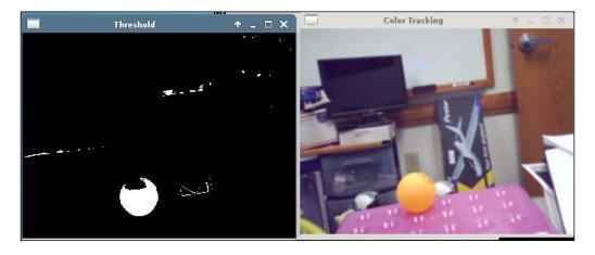
Notice the white pixels in your threshold image showing where the ball is located. You can add more OpenCV code that gives the actual location of the ball. You can actually draw a rectangle around the ball in your original image file as an indicator of the location of the ball. Edit the camera.py file to look like the following screenshot:
