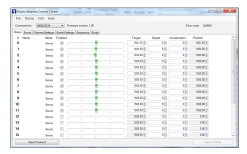
Now you can use the sliders to actually control the servos. Check that servo 0 moves the right front lower servo, servo 1 moves the right front middle servo, servo 2 moves the right front upper servo, and so on. You can also use this to center the servos. Set all the servos such that the slider is in the middle. Now unscrew the servo horn on each servo until the servos are centered at this location. At the zero degree location of all servos, your quadruped should look like this:
