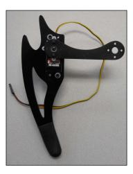
3. Complete the leg by connecting two of the servo brackets together at right angles, mounting the HS-645MG on one of the brackets, and then connecting this servo to the interconnect piece, like this:
