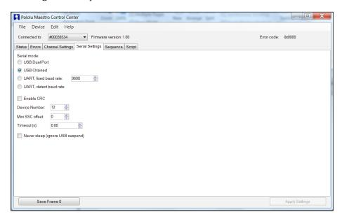
Make sure that **USB Chained** is selected; this will allow you to communicate with and control the motor controller over USB. Now go back to the main screen by selecting the **Status** tab, and now you can actually turn on the 12 servos. The screen should look like this screenshot:
