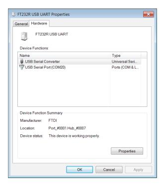
Note that the device is connected to the **COM20** serial port. We'll use this to communicate with the device and configure it. You can use any terminal emulator program; I like to use PuTTY, which is already on my computer. It is free and available at http://www.chiark.greenend.org.uk/~sgtatham/putty/download.html.
