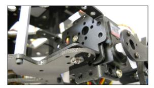
8. Now connect the other servo to the empty servo bracket and the body, like this:
