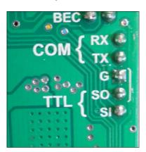
3. Now connect the green cable to the SI connection, the white cable to the SO connection, and the black cable to the G connection. Here is an image of what it should look like:
