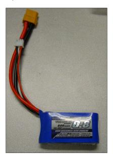
You'll also need a USB battery to supply the BeagleBone Black with power. You can connect the servos to the power of this LiPo battery by using male-to-male solderless wires. The red wire output of the LiPo battery will be 7.4 volts, and the black wire output will be GND. Here is an image of these connections:
