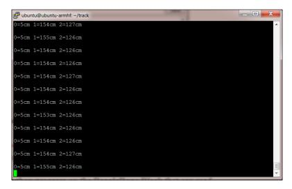
Now you can use the sonar sensors to detect objects both in front and on each side of your robot.
