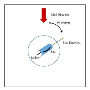
The problem with this is, if you sail in this direction, you cannot reach a destination that is less than 60 degrees in the wind direction. To reach destinations in this area, you'll need to do a manoeuvre called a **tack**. To tack is simply to use a set of manoeuvres, crossing back and forth at a 60 degree angle into the wind, so that you can arrive at a destination that is directly against the direction of the wind. Here is a diagram of tacking:
