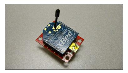
The advantage of using this device is that it is configured to make it very easy to create and manage a simple link between two XBee series #1 devices. Make sure that you have an XBee device that supports ZigBee series #1. You'll also need to purchase a shield that provides a USB port connection to the device. Note that some USB XBee shields require a special driver to talk to the device; check yours when you purchase the device.
