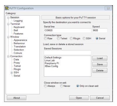
2. Configure the terminal window with the following parameters (the **Serial** option on the **Category** option set): insert 9600 in the **Speed (baud)** field, insert 8 in the **Data bits** field, select **None** from the **Parity** drop-down menu, and insert 1 in the **Stop bits** field.
