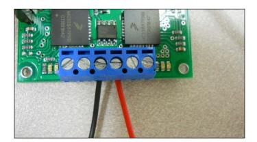
3. Now connect one of the motors to the motor controller by connecting the red and black wires with male connectors to the two outer blue screw connectors, the red one to A and the black one to B using the male to male jumper wires. The connection to the motor controller should look like this:
