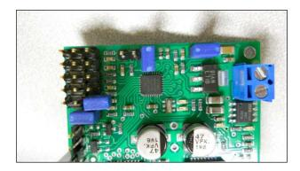
You should supply the unit with power by making sure you have batteries in the battery holder. Now that you have your basic motor controller functionality up and running, you need to connect the motor controller to the BeagleBone Black. Plug the USB cable that you just connected to the motor controller to the BeagleBone Black.
