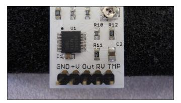
You'll need a **GND** and **+V** connection. The **+V** pin will be connected to the 5-volt connection of the BeagleBone Black, P9\_5 of the GPIO set, and the **GND** pin will be connected to the ground connection of the BeagleBone Black ADC, P9\_34. The **TMP** pin on this sensor is a temperature measurement – you won't use it in this project.
