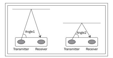
The different angles give you an indication of the distance to the object. Unfortunately, the relationship between the output of the sensor and the distance is not linear, so you'll need to do some calibration to predict the actual distance and its relationship to the output of the sensor. You'll learn more on that later.
