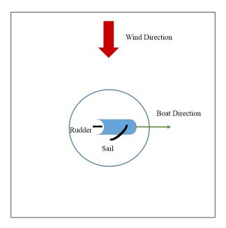
This is called a **beam reach**, and once you have made any turn, you'll adjust your rudder to be straight behind the boat again. The sail will be out at about 45 degrees, or half way between in line with the bow and stern, and all the way to the side.
