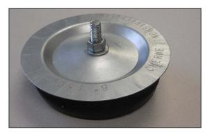
The concept of the plug is quite simple. As you tighten the nut, the rubber seal spreads and seals the PVC pipe.
