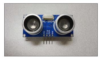
This particular sensor does not have a USB interface but only four pins, one each for **5V**, **GND**, **Trig** which sends a sonar pulse, and echo which receives the sonar pulse. One alternative is to connect your sensors to the BeagleBone Black since it has GPIO pins.
