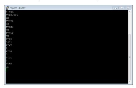
The **OK** response comes back from the device as you enter each command. Now plug the other device into the PC. Note that it might choose a different COM port. Go to the **Devices and Printers** section, double-click on the device, and select the **Hardware** tab to find the COM port. Follow the same steps to configure the second device, except that there will be two changes. Here is the terminal window for these commands:
