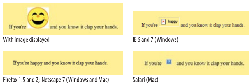
Figure 7-3. Most browsers display alternative text in place of the image (either with an icon or as inline text) if the image is not available. Safari for Macintosh OS X is a notable exception.
