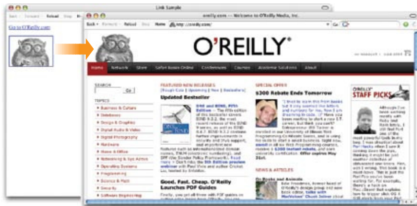
Figure 6-1. When a user clicks on the linked text or image, the page you specify in the anchor element loads in the browser window.
