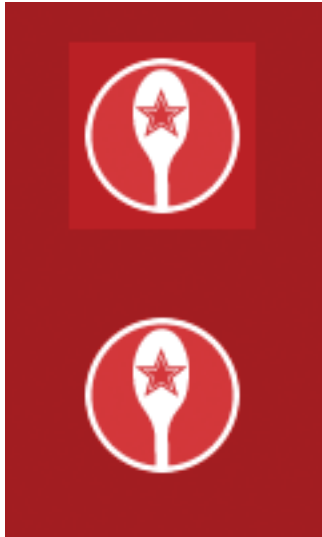
Figure 3-11. On 16-bit monitors, RGB colors get shifted around. In this figure, although the graphic in the foreground uses the identical RGB values as the color in the background, you can still see the outline of the image on the page (top). The only way to fix this is to make the image transparent and allow the background to show through (bottom).
