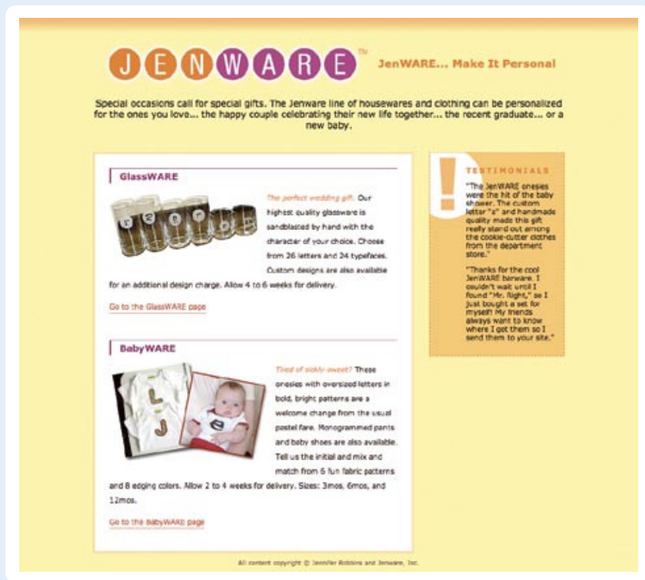
Figure 15-9. A new two-column layout for the JenWARE home page, created with a float and a wide margin on the following content.
