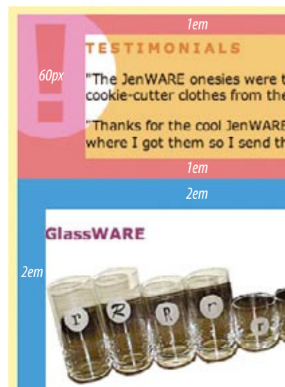
Figure 14-8. The pink area indicates padding added to the testimonials section. Blue indicates the products section padding.
