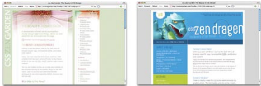
Figure 3-8. The design on the left ( Faded Flowers by Mani Sheriar at csszengarden.com ) uses a fixed-width page positioned on the left. When the browser window is resized larger, the extra space is added to the right of the page. The page on the right ( Dragen by Matthew Buchanan, also at CSS Zen Garden ) has the fixed-width page centered in the browser window. Extra space is split on the left and right margins.
