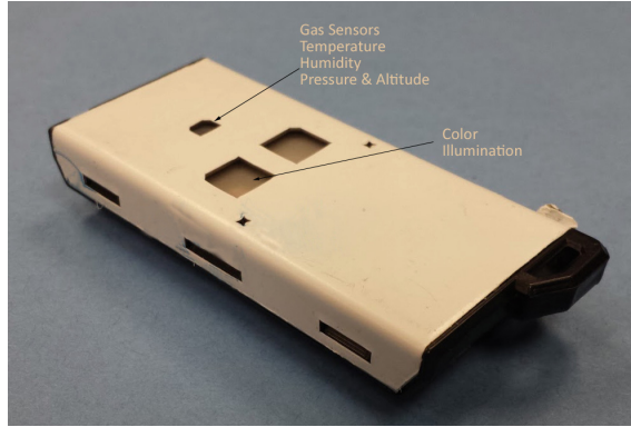
Fig. 3. Sensordrone device with different sensors (ambient temperature, precision gas, humidity and altitude are utilized in this paper). Device dimensions: 2.67 \times 1.10 \times 0.49 inch 3 .
