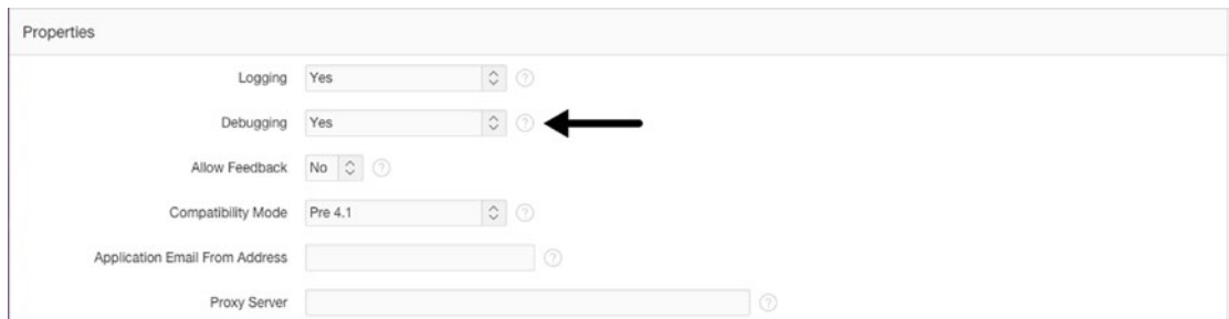
Figure 7-5. The Properties region of the application definition where interactive debugging is enabled or disabled
