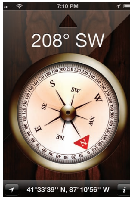
Figure 6.1 iOS 6's Compass app was skeuomorphic; it resembled its real-world counterpart, making the program easily understandable to users.
