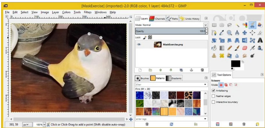
Figure 7-12. To extract an object from an image, open the image, select the Scissor tool, and click on its edge. Clicking it a second time enables edge detection
