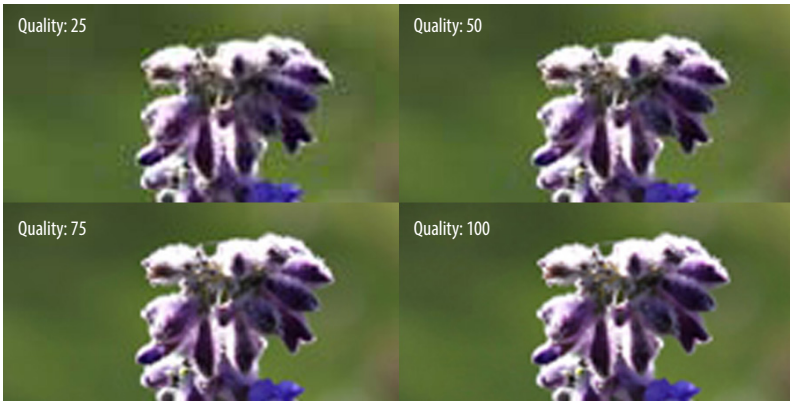
Figure 3-2. In this comparison of Photoshop’s Save for Web export quality, the lower-quality JPEG images have more artifacting around edges of high contrast, such as the green background surrounding the top white leaves.
