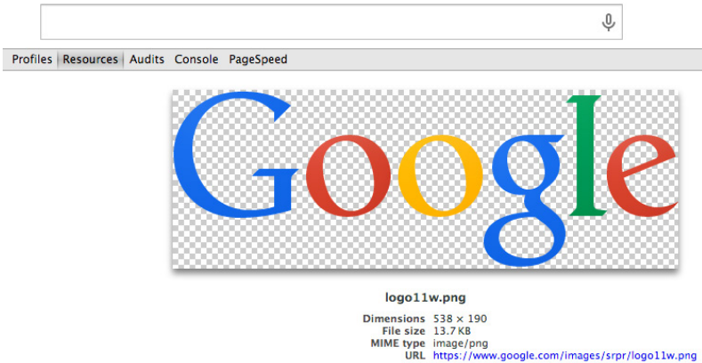
Figure 5-1. In this example, we can see that the size at which the Google logo is displayed is smaller than the actual size of the logo file.
