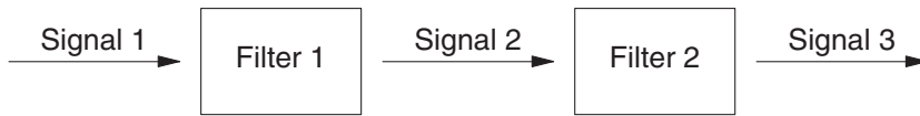
FIGURE 4-11. A filter chain: each filter applied to a signal yields another signal, which itself can be filtered.
