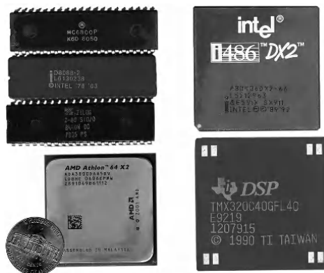
Figure 1.11. A few old microprocessors: (a) Motorola™ 6800 (1974, \approx 6,800 transistors), Intel™ 18088 (1979, \approx 29,000 ), Zilog™ Z80 (1976, \approx 8,500 ), AMD Athlon 64X2 (1999, from \approx 122 millions to \approx 243 millions); (b) Intel i486 DX2 (1989, \approx 1.2 million), Texas Instruments™ TMX320C40 (1991, \approx 650,000 )
