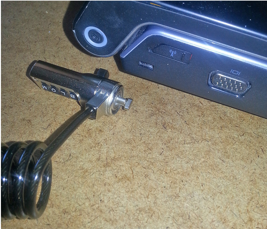
FIGURE 9-1 A typical cable lock uses the K-slot on a notebook.
