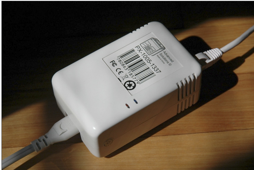
FIGURE 7-7 The Pwn Plug looks like a common power adapter.
