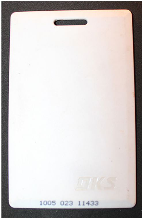
FIGURE 6-16 A traditional proximity card is the size and shape of a credit card.
