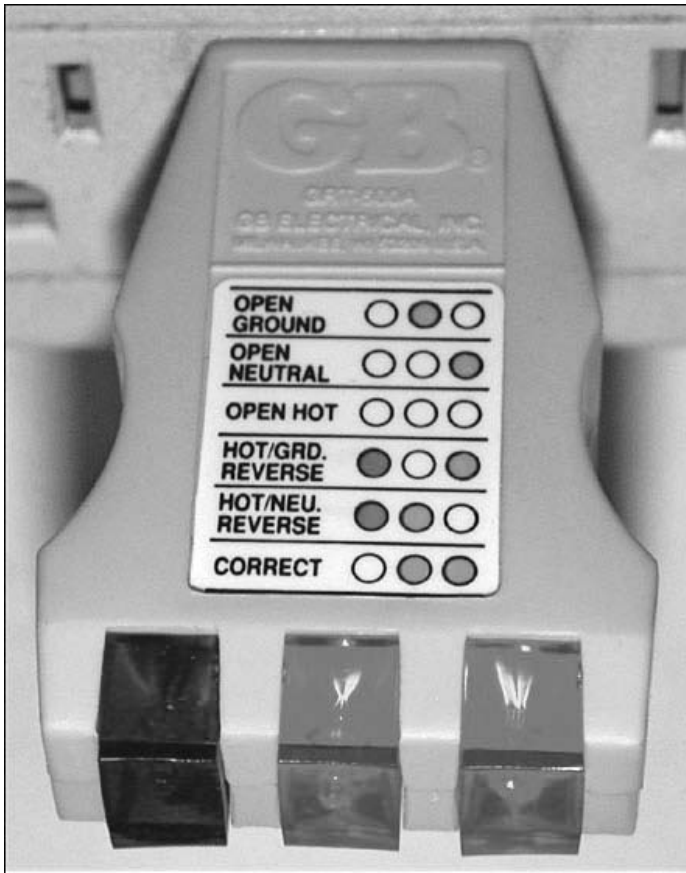
Figure 4-16 An outlet tester like this one can find wiring problems quickly. This outlet is wired correctly.
