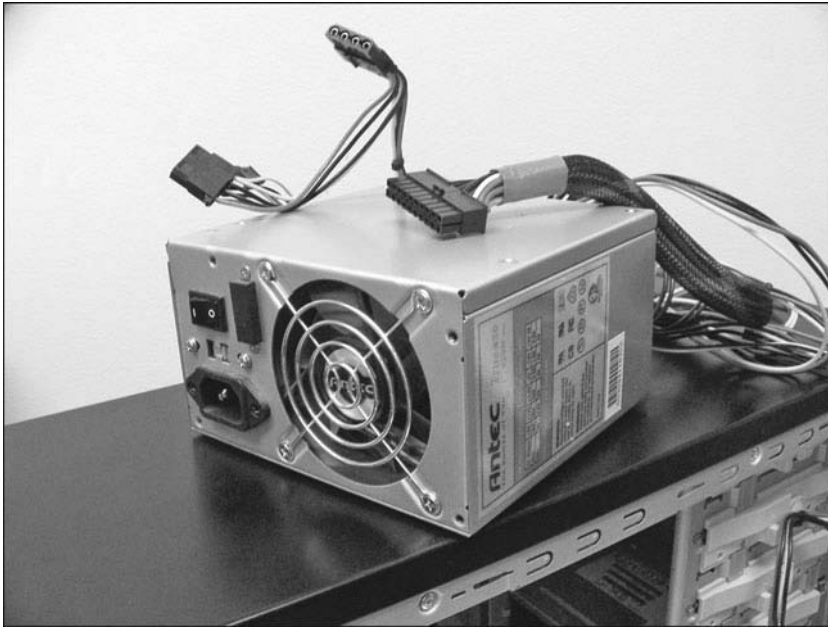
Figure 4-1 A typical ATX power supply.
