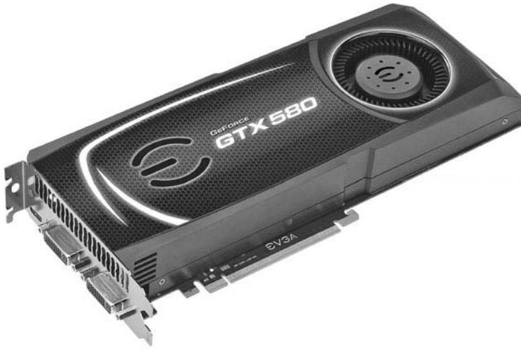
Figure 4-20 The EVGA GeForce GTX 580 is a high-performance PCI Express x16 video card that requires a two-slot fan shroud. Image courtesy of EVGA Corporation.
