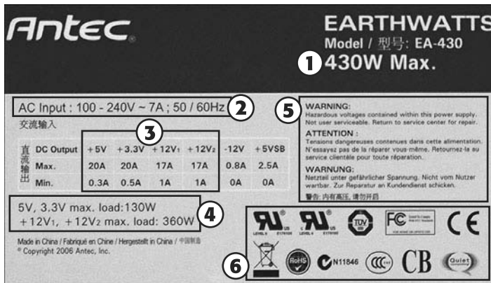
Figure 4-2 A typical power supply label.
