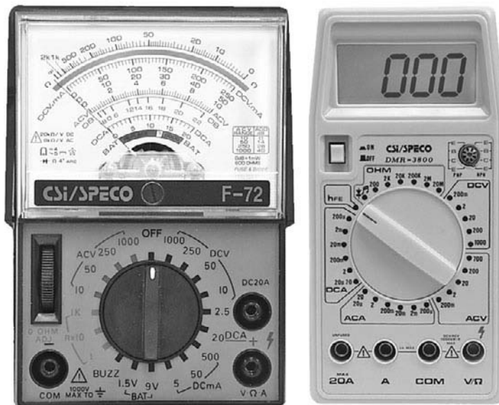
Figure 4-13 Typical analog (left) and digital (right) multimeters. Photos courtesy of Colacino Electric Supply, Newark, NJ.
