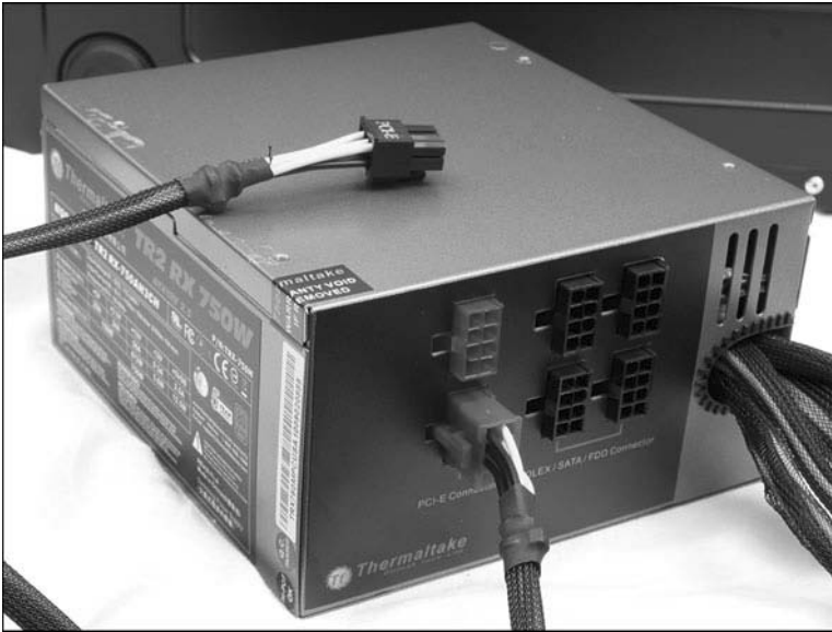
Figure 4-7 A modular power supply includes cables you can attach to customize support for your system's needs.
