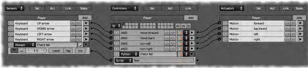
Figure 11–22. You do not need an actuator to call Python scripts. It is done in the controller.
