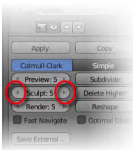
Figure 3–31. Multiresolution level control. Using the arrows at either end, you can tweak how smooth the multiresolution levels are.
