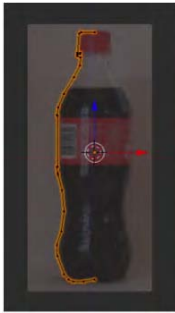
Figure 6–30. Tracing and extruding a single vertex to outline half a bottle for spinning
