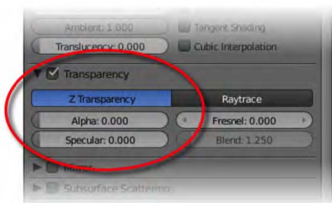
Figure 10–21. Enabling transparency settings. Don't forget to slide the Alpha and Specular levels down to zero.
