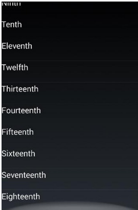
Figure 5-11. ListView scrolls automatically when there are more rows than fit on the screen
