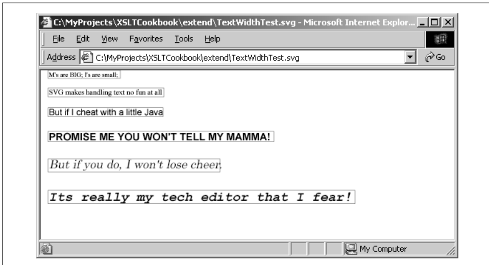
Figure 14-1. Creating correctly sized text-bounding rectangles with the SVGFontMetrics extension
