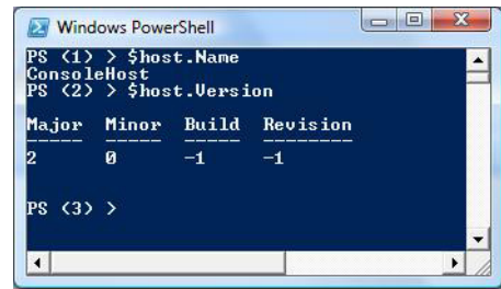
Figure 10.2 You can see the host name and version properties for the PowerShell console host.
