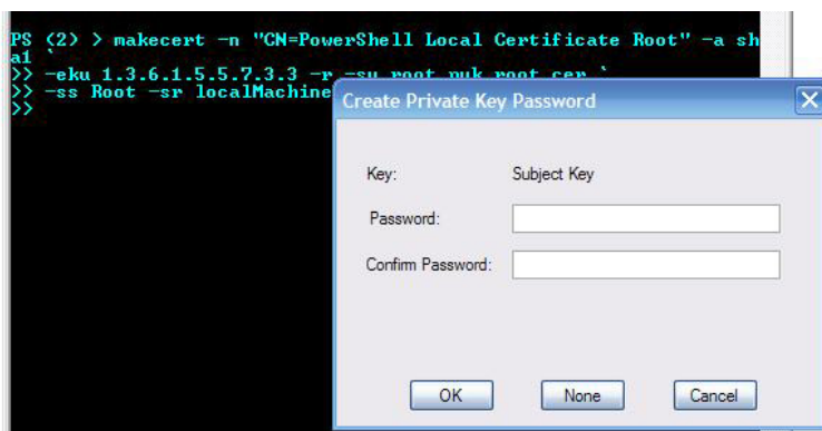
Figure 21.3 What you see when you run makecert to create the self-signing authority
