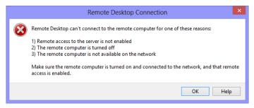
FIGURE 7-3 Access denied when attempting to connect to Remote Desktop.
