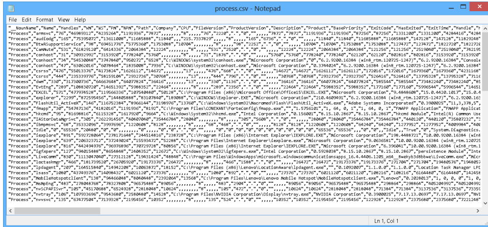
FIGURE 5-7 Opening a .csv file in Notepad is not the best use of the file format due to the numerous commas and quotation marks in the file.
