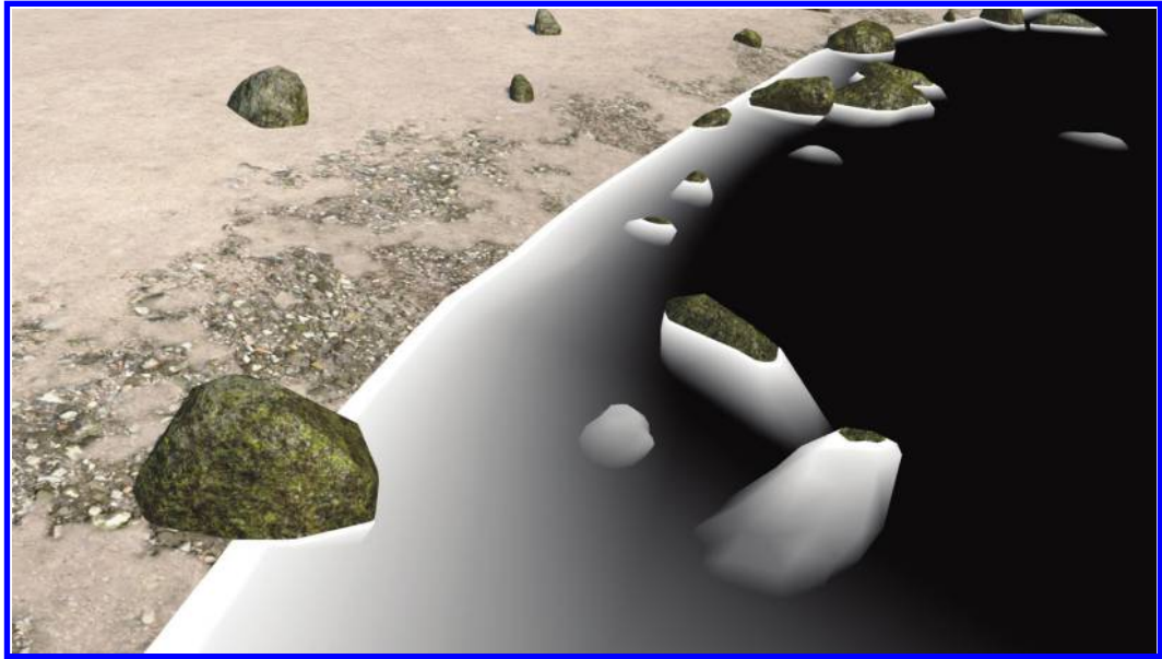
Figure 11.13 Depth-based foam factor.
