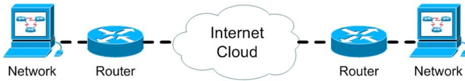
Figure 12.5. Router connections to the Internet cloud
