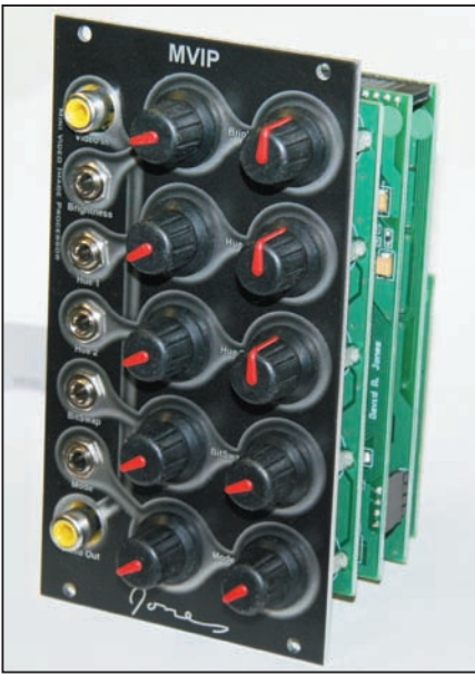
Color Plate 32. The MVIP (Mini Video Image Processor), designed by Dave Jones, is less than three inches wide (2011). (photo & courtesy. Dave Jones Design).
