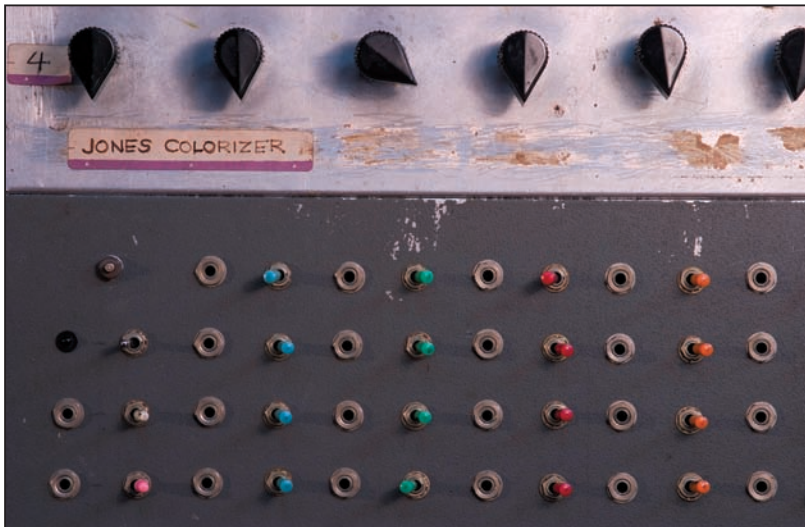
Color Plate 37. Detail of the first Jones Colorizer by Dave Jones, built at the Experimental Television Center. Control panel above, main unit with control voltage inputs below (c. 1974/75). (photo. Olivia Robinson. courtesy. Experimental Television Center).
