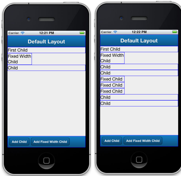
Figure 4.6 The result of a simple default layout. The left side shows the initial state of the code from listing 4.3, whereas the right side shows the result of clicking the Add Child and Add Fixed Width Child buttons a few times. The blue border makes it easier to see the bounding boxes for each item.
