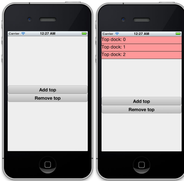
Figure 5.5 The initial results of listing 5.2 (left), and the same after adding the top docked container by tapping the button a few times (right)
