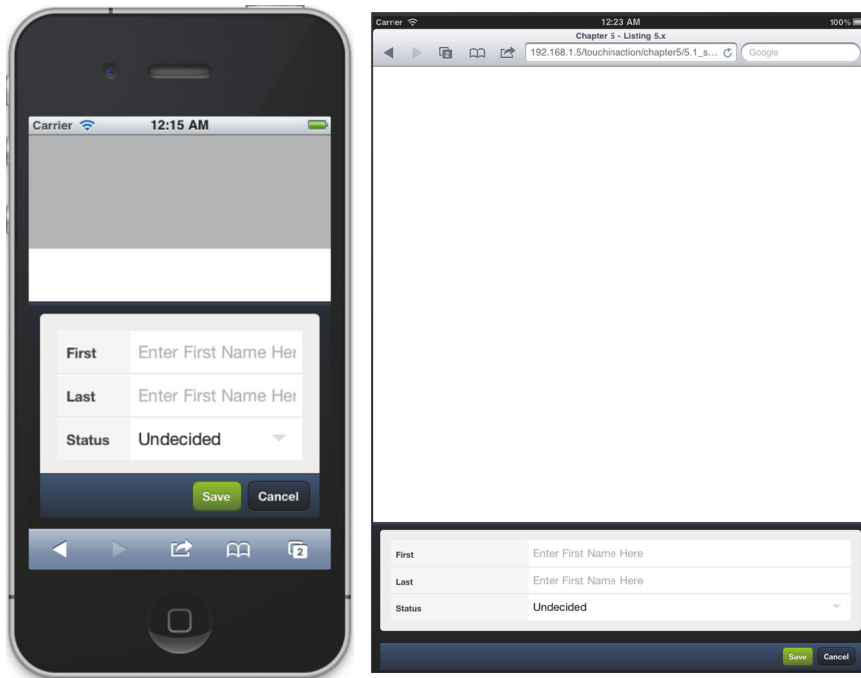
Figure 6.2 A sheet sliding in from the bottom on a phone (left) and the same sheet rendered on a tablet (right)
