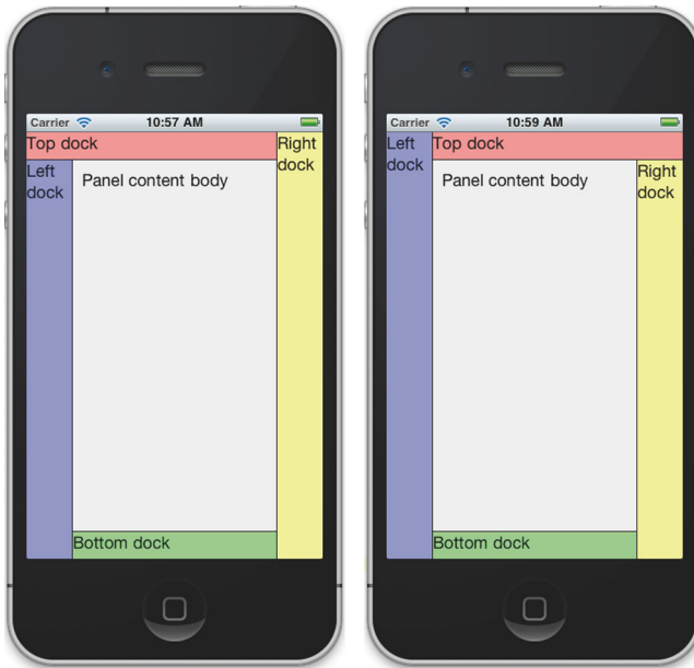
Figure 5.2 The order in which you place docked items will affect the amount of screen space they have.
