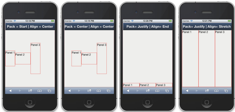
Figure 4.10 Mixing the pack parameter with different align options can produce interesting and useful combinations.
