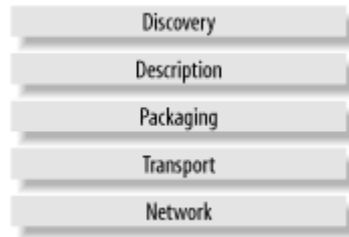
Figure 1-5. The web service technology stack
