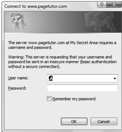
Figure 17-5. Internet Explorer shows this password prompt when a page requiring authentication is requested.
