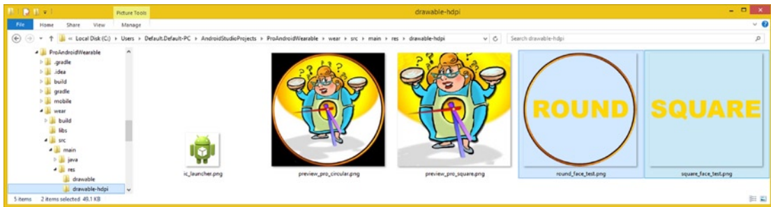
Figure 11-38. Add test bitmaps into the wear/src/main/res/drawable-hdpi folder using an OS file management utility
