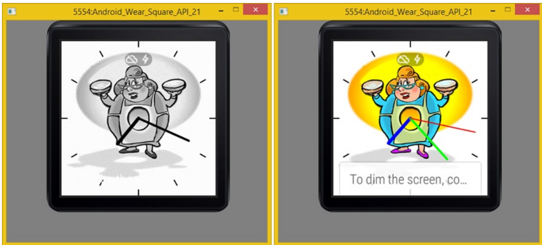
Figure 12-22. Use Settings ► Change watch face ► Pro Watch Face series, and F7 to test ambient mode
