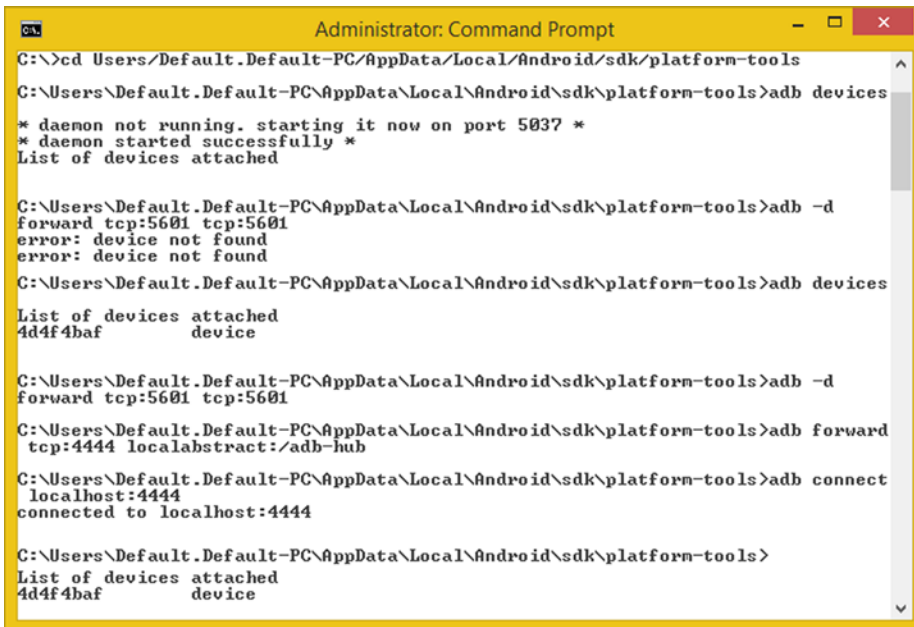
Figure 15-30. Use ADB commands to set up the USB smartphone connection and smartwatch Bluetooth
