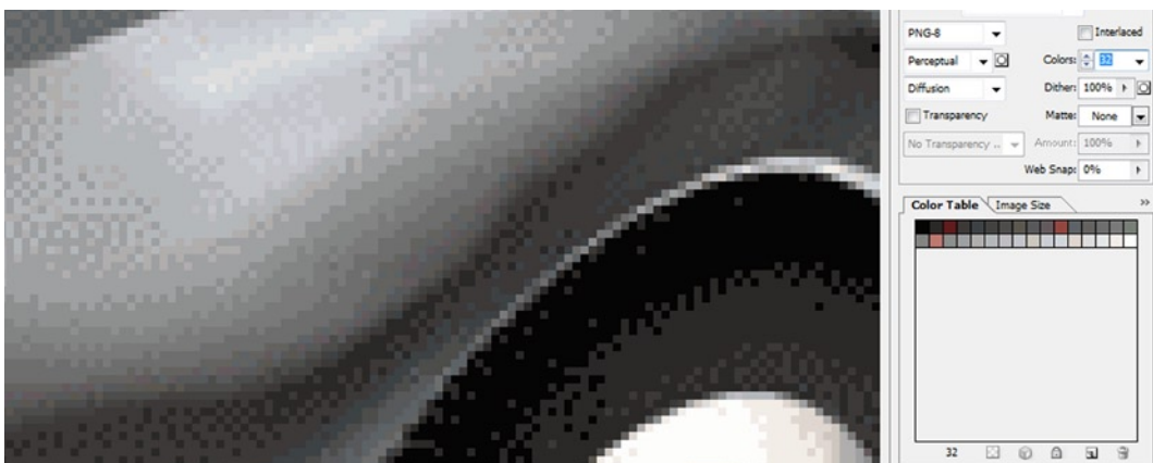
Figure 6-3. Showing the dithering effect in an indexed color image with compression set to 32 colors (five-bit color)
