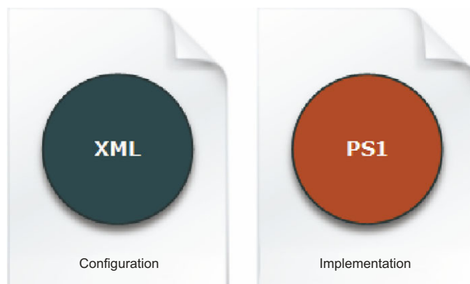
Figure 10 Separating configuration-specific details from a script's implementation and execution is more complicated up front, but makes both easier to maintain.
