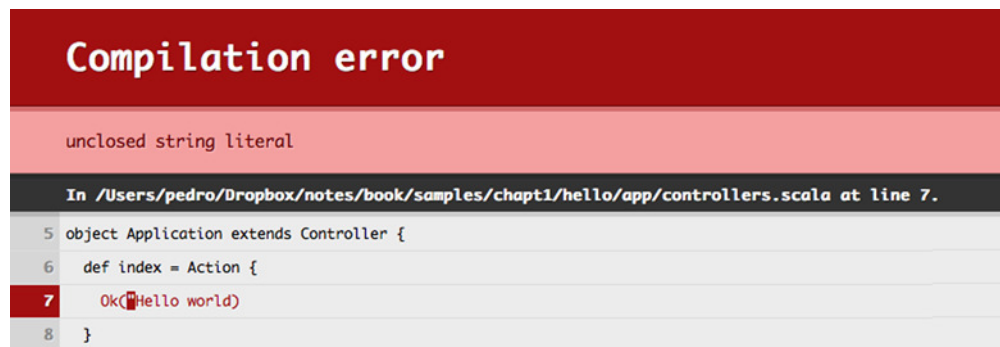
Figure 1.4 Compilation errors are shown in the web browser, with the relevant source code highlighted.
