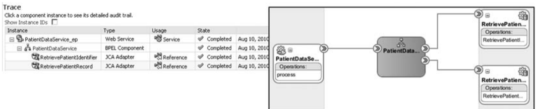
FIGURE 5-23. Fusion Middleware Control—SOA console’s overview of the flow of messages resulting from a single service call
