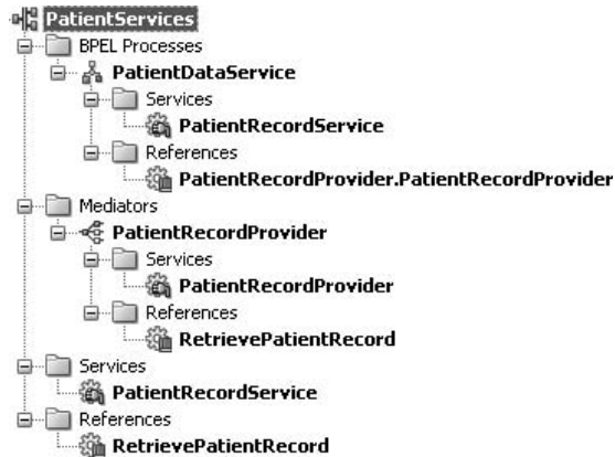
FIGURE 14-2. Composite Editor showing the structure of the composite in a tree view
