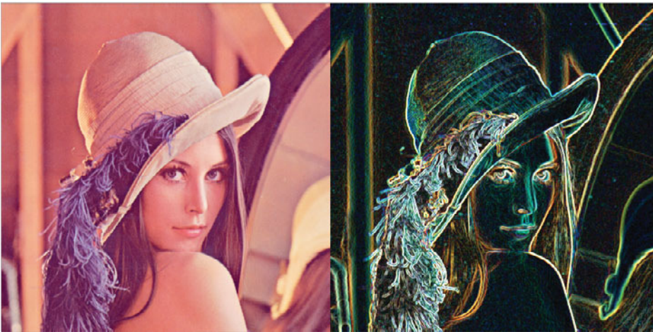
Figure 15.1 OpenCL Sobel kernel: input image and output image after applying the Sobel filter
