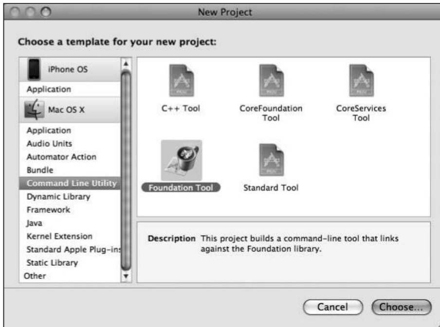
Figure 2-1. Making a new foundation tool
