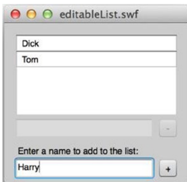
Figure 9-18. An example of multiple components working together to create a simple interface
