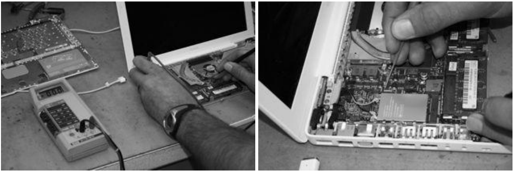
Figure 3.8: One way to see if a piece of computer hardware is working is to connect a set of probes to a meter (left) and then use the probes to measure signals coming from the CPU or other parts of the system (right). The RubyLabs module has a number of “software probes” that will be used to monitor the execution of sieve and other methods.
