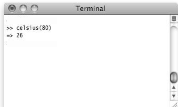
Figure 2.3: A terminal emulator application allows us to run software with a command line interface. The first line shown here asks Ruby to compute the Celsius equivalent of 80°, and the second line is the output.
