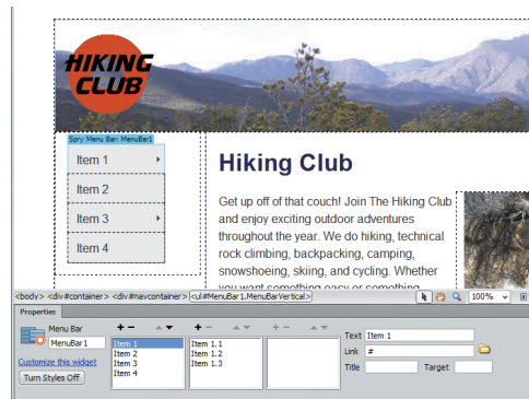
B The brand-new Spry menu bar on our page starts off with some default values.
