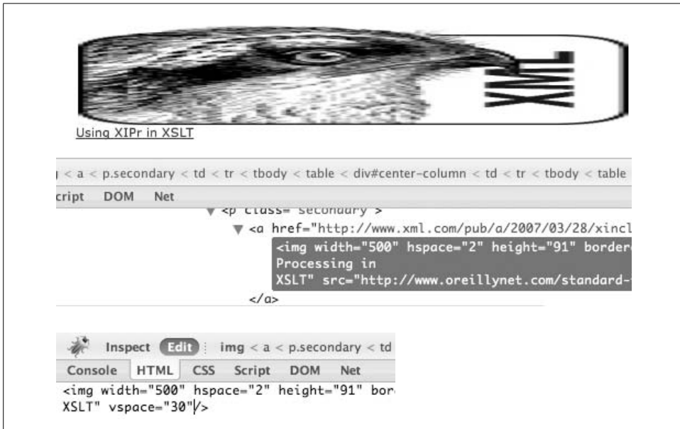
Figure A-5. You can use Firebug to hack on the HTML in the page and see live results
