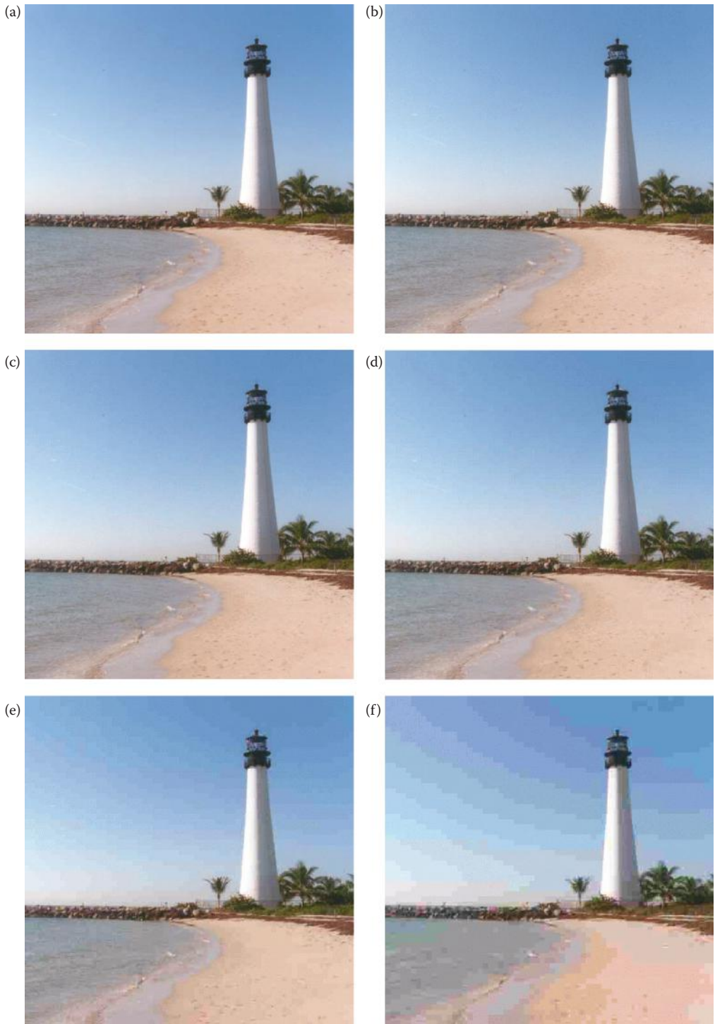
FIGURE 10.3-21 The original DCT-based JPEG algorithm applied to a color image. (a) The original image, (b) compression ratio = 34, (c) compression ratio = 58, (d) compression ratio = 80, (e) compression ratio = 131, (f) compression ratio = 201.
