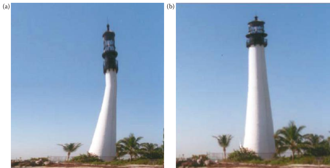
FIGURE 1.3-3 Geometric distortion correction (a) distorted image, (b) restored image (note the process is not perfect).
