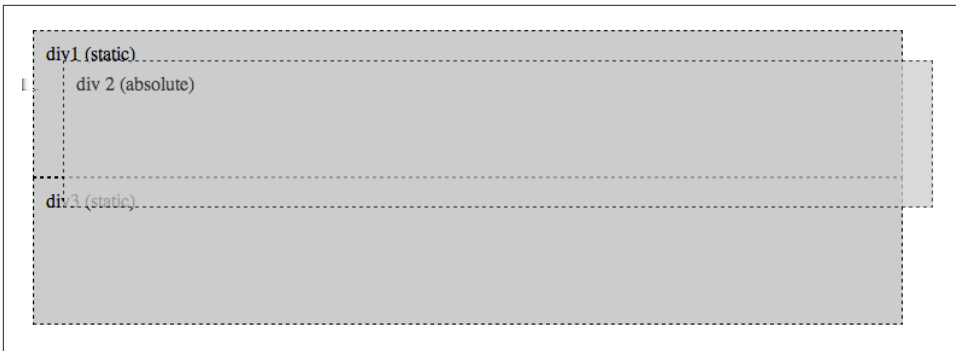
Figure 3-4. An absolutely positioned element with an opacity of 0.75 and top and left values of 75px—note that the space it would have occupied in the normal flow collapses
