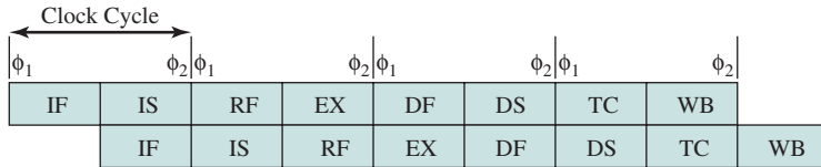
(b) R4000 pipeline
