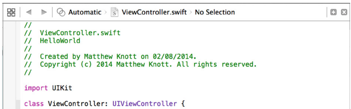
Figure 2-13. The jump bar in the Assistant Editor shows which file is open
