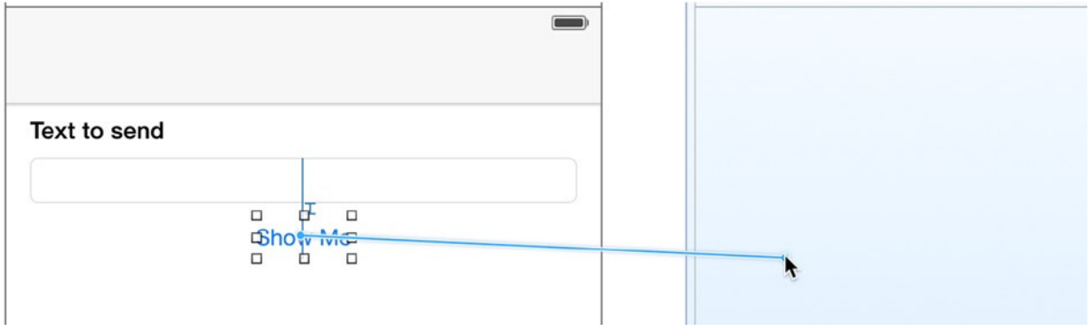
Figure 3-26. Making a connection from the Show Me Button to the second view controller
