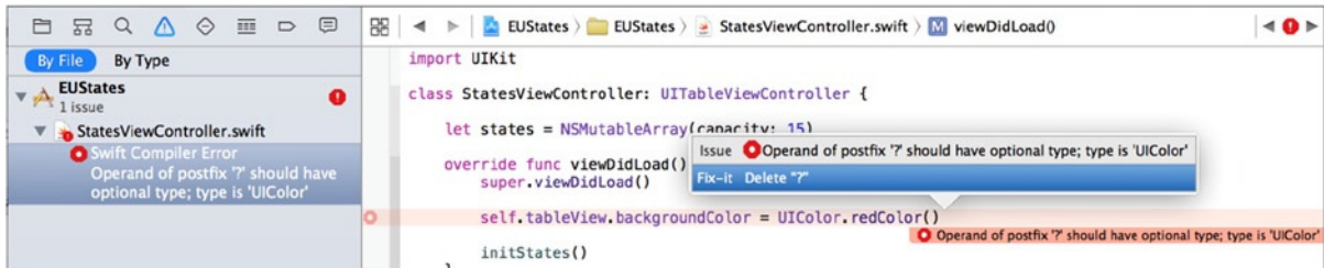
Figure 11-29. The issue detail pop-over, explaining the issue and offering to fix it
