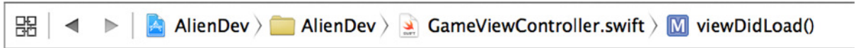
Figure 10-15. The jump bar is located at the top of the code window
