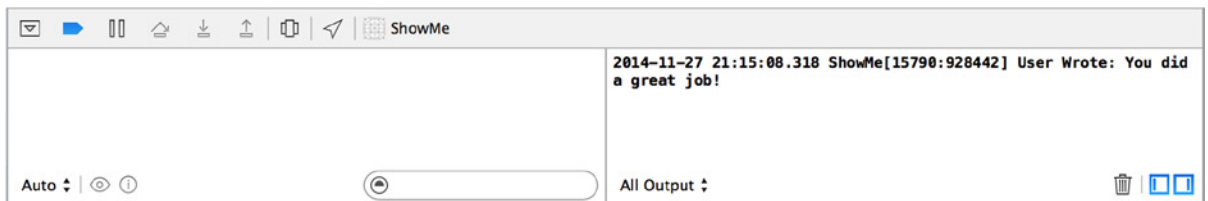
Figure 3-31. The result of the NSLog method call is displayed in the output console
