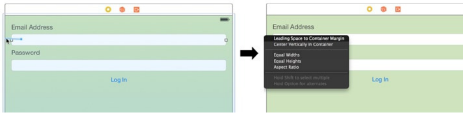
Figure 6-13. Dragging a line from the text field to the side of the view (left) presents a context menu (right)
