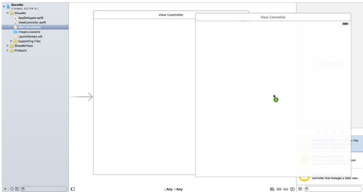
Figure 3-14. Dragging a view controller from the Object Library to the design area
