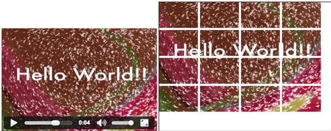
Figure 5-5. Tiling a video into a canvas in Chrome, video on left, canvas on right
