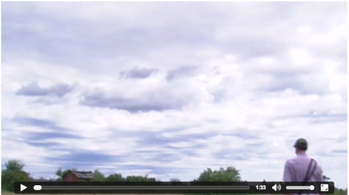
Figure 2-7. The @controls attribute, shown here in Chrome, adds user controls to a video
