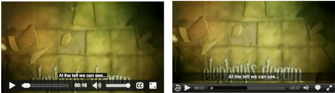
Figure 4-6. Video element with @default activated track child element in Opera (left) and Safari (right)
