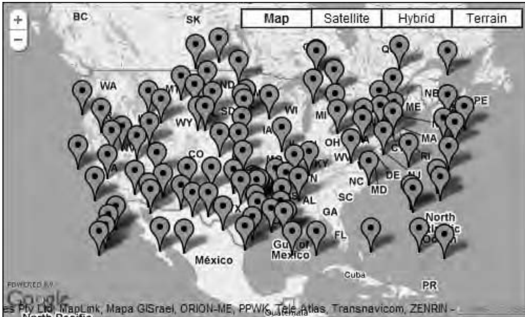
Figure 9-12. 100 markers are added to the map. The MarkerManager library only displays those that are within the current viewport.
