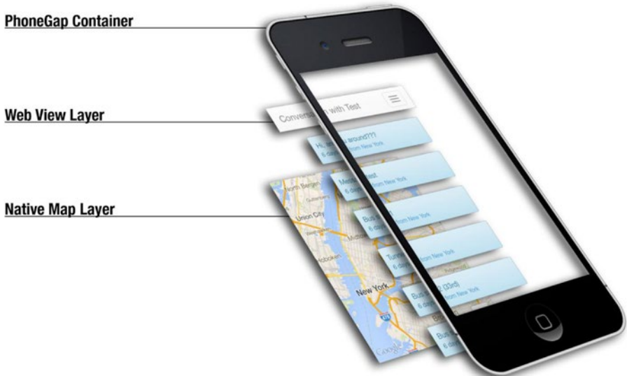
Figure 10-3. The native map layer will be positioned behind your web view (for example, the conversation template). Solid elements will overcast the map
