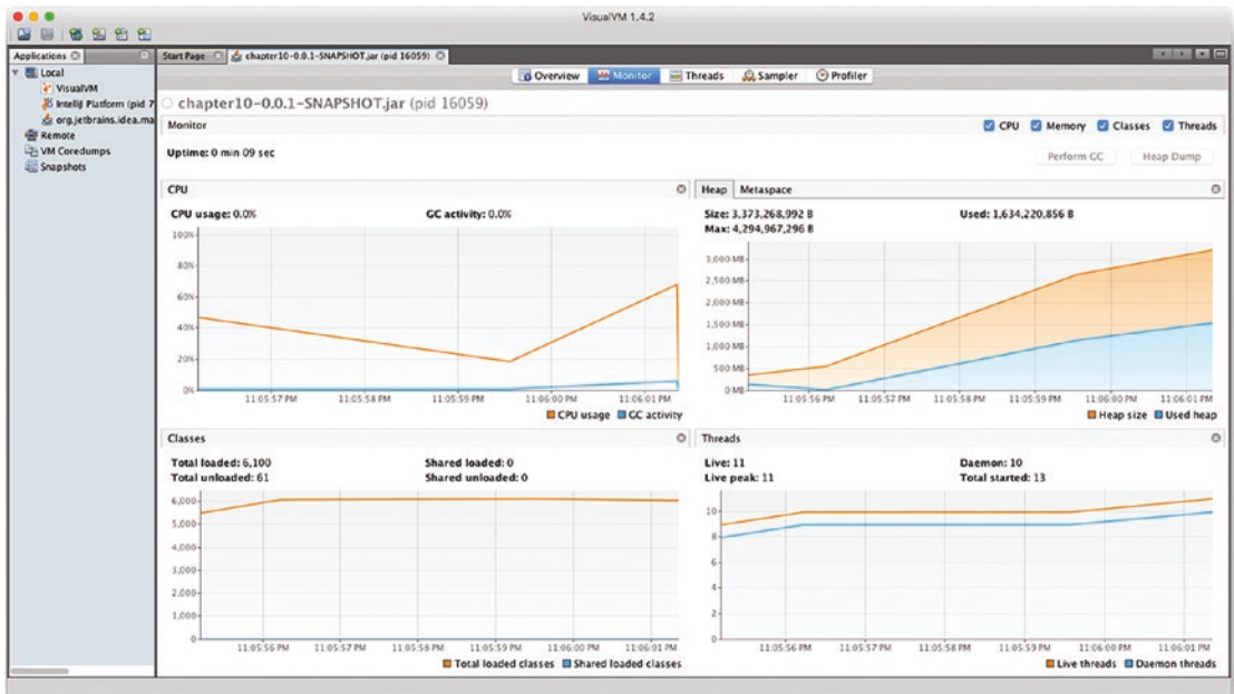
Figure 11-10. Monitoring results of the statement job with a memory leak
